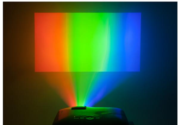
Projector brightness is measured in ANSI lumens, with corporate units typically ranging from 3,000 to 6,000 lumens or more. The higher the brightness, the easier the image will be to see, especially in a large room with significant ambient light.
