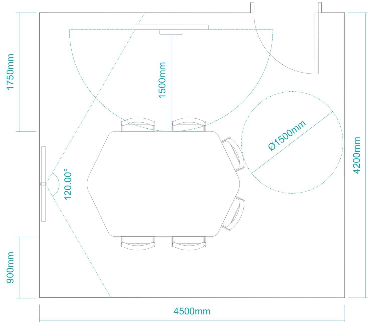
**Key Hint:** Make use of asymmetry in a room when looking to feature a jamboard, to maximise space efficiency. In this case, only the jamboard side of the room needs to be accessible.
