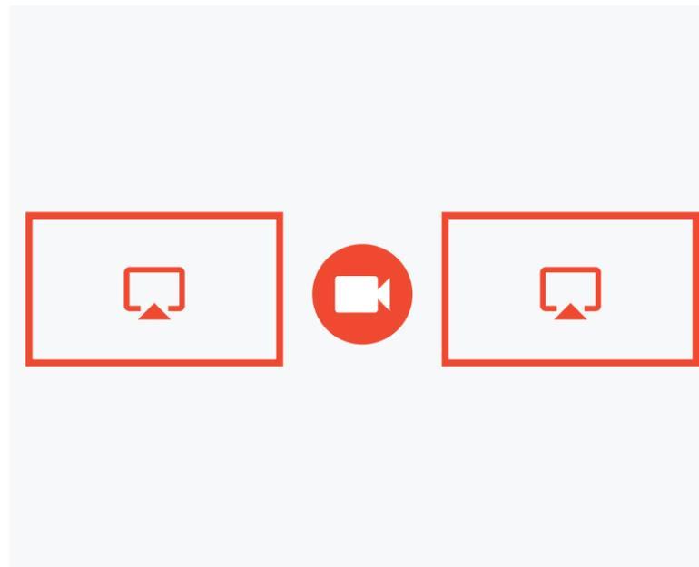
In dual screen setups the camera is usually best mounted between the screens and kept central to the table.
