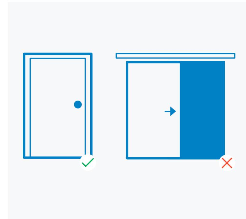
Doors are generally the acoustic weak link as sound is able to go through and flank around the door through the gaps in the doorway. Insulated metal doors are preferred, followed by solid wood doors. Generally swing doors perform better than sliding doors. Perimeter acoustic seals will aid the sound separation performance and should be considered for any meeting room.
