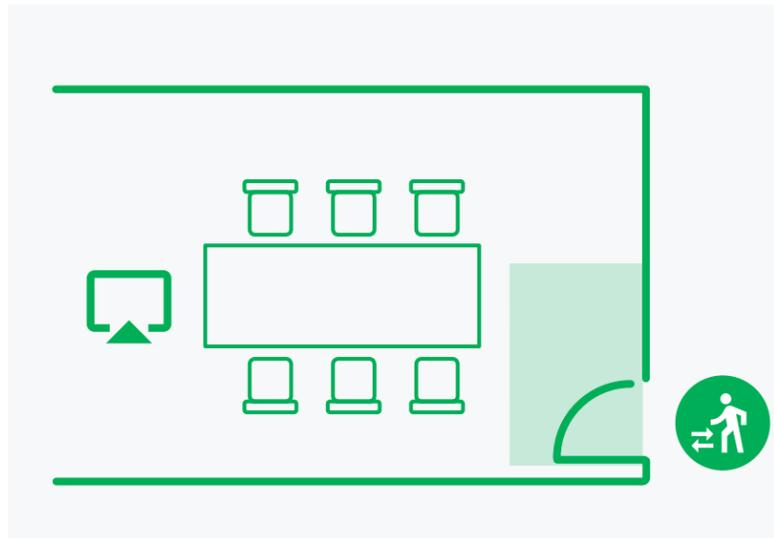
Consider how you might arrive into the space before and during meetings. A well placed entry point opposite the screen wall and away from the table will minimise disruption. Maneuvering clearance is also required at the doorway as per local code and specified by architect.
