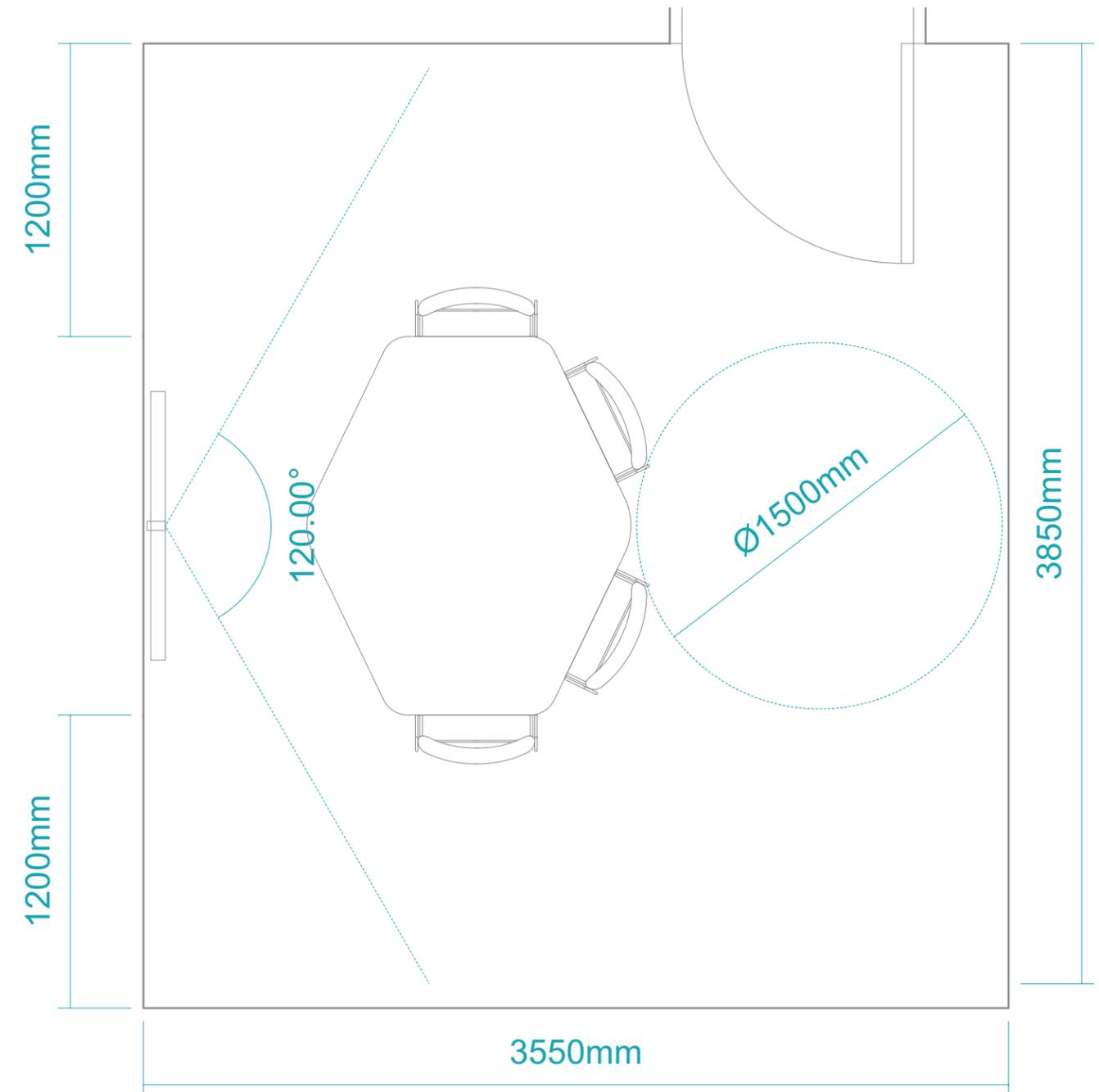
**Key Hint:** Clear access and wheelchair turning space are just as much needed in the smallest rooms as they are in the larger spaces.
