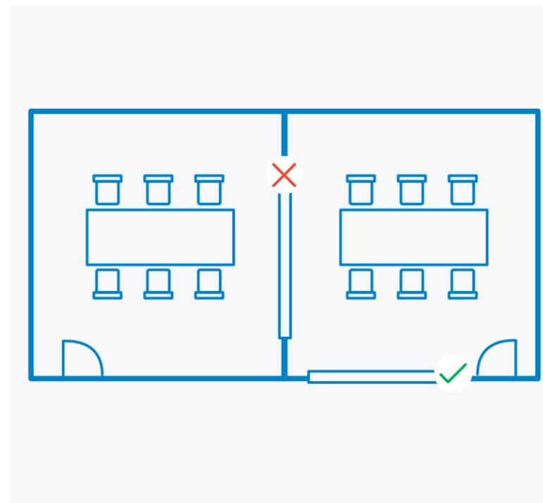
Use of glazing is great for open plan office spaces, but be warned of its inferior acoustic compared to plasterboard walls. Aim to limit glazing to the wall with the entry door, and avoid placing glazings between meeting rooms.
