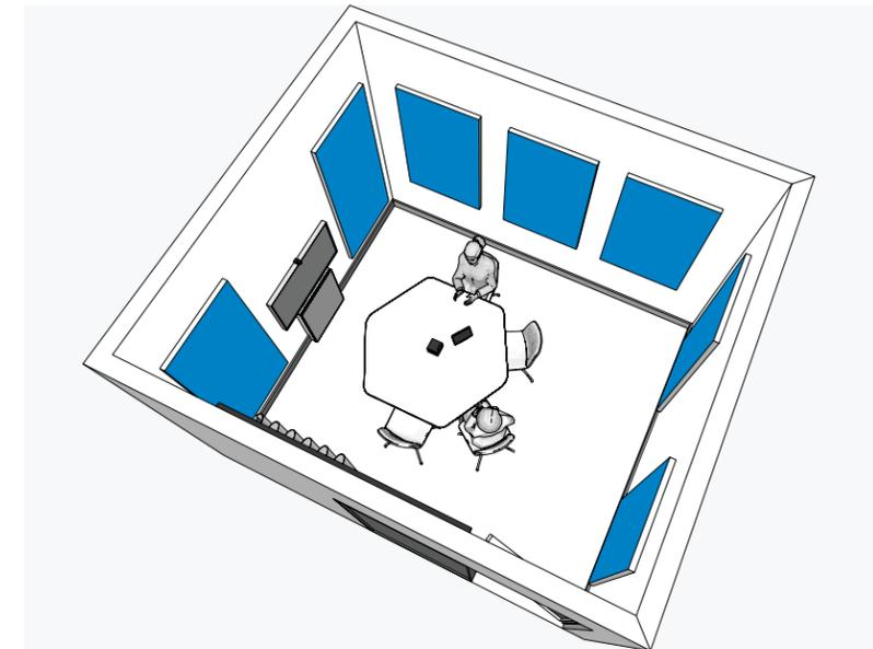
Wall treatment should ideally be placed at seating head height approximately 1m from the floor, up to the ceiling.
