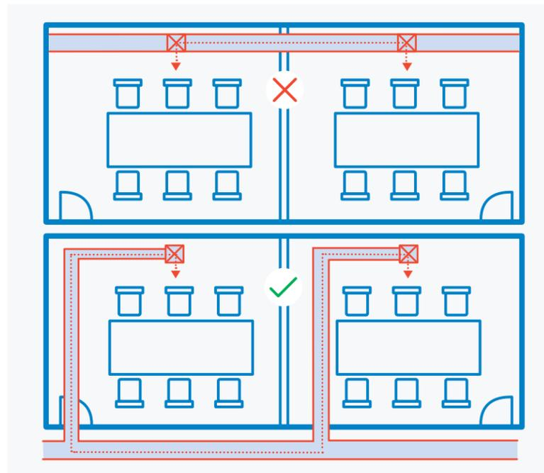
Short ductwork between spaces are a common cause of unwanted sound transmission. When designing new spaces consider duct routing to minimise this concern.
