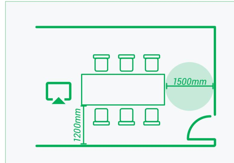
Ensure there is at least 1200mm clearance around fixed furniture for accessibility, this is greater than most local codes to provide good accessibility. A turning circle of at least 1500mm must also be provided between the table and the rear wall.
