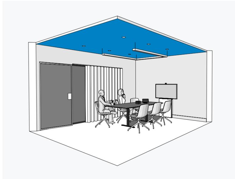
Ideally the entire ceiling should feature acoustic treatment to at least NRC 0.7. Suspended ceilings (ACT), are the most common solution, but other solutions such as suspended fabric wrapped panels or an acoustic spray treatment could also be considered.
