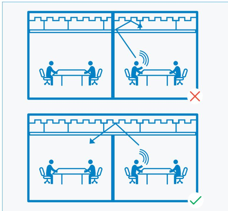
Partitions should be full height. Half height partitions allow for sound to transfer over the wall and limit sound isolation.
