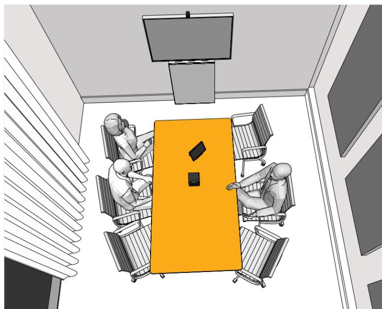
Table legs must not restrict seating or leg movement. Compartments for AV equipment and user-accessible cables can be incorporated into the tabletop to assist participants using small devices.
