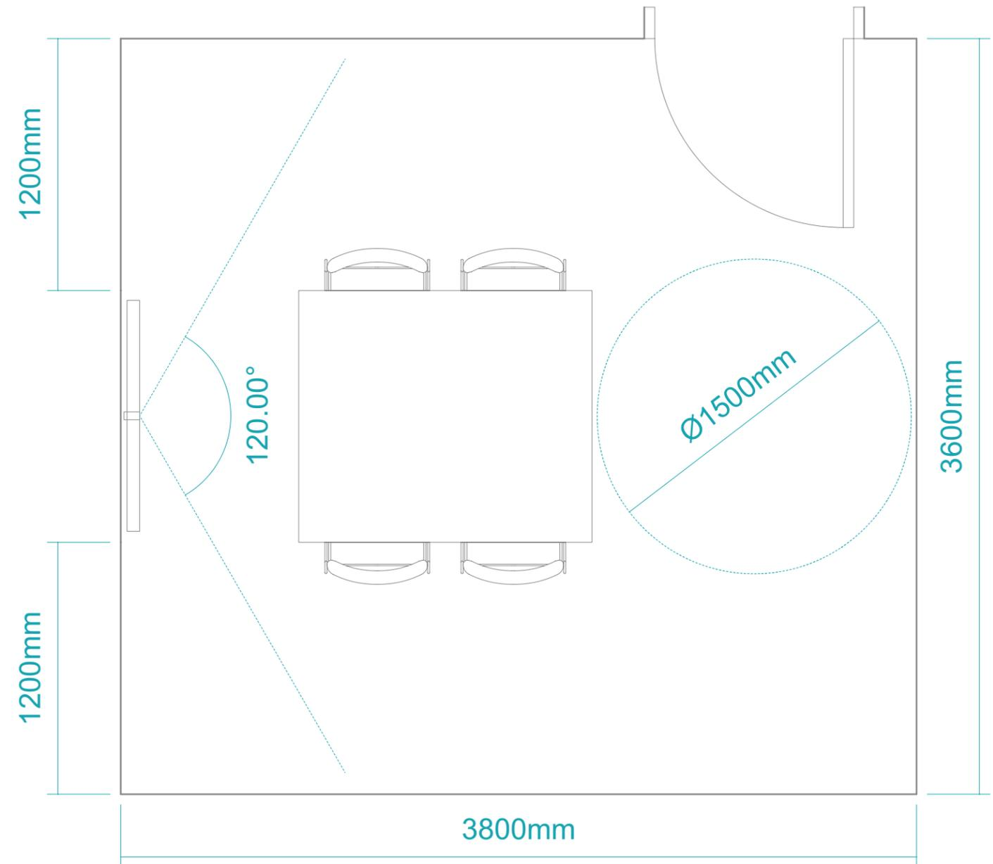
**Key Hint:** Clear access and wheelchair turning space are just as much needed in the smallest rooms as they are in the larger spaces.
