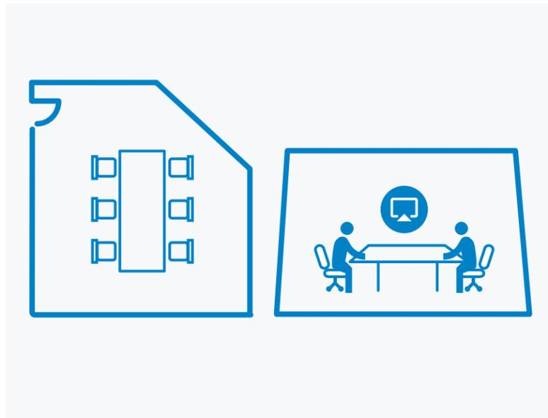
You can look to take advantage of unusually shaped spaces—angled, or non parallel walls can provide acoustic benefits. However this is purely secondary gain and not a design requirement.
