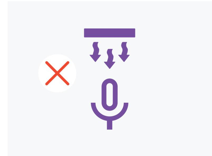
Avoid locating intake or extract (supply/return) ductwork above or near sensitive GVC equipment such as microphones. Unwanted noise from air flow on microphones can cause disruptive noise on the video call.
