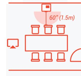
This is the recommended space around the Jamboard to allow effective collaboration. The smallest recommended zone is a semi circle of radius 60" (1.5m) in front of the Jamboard.
