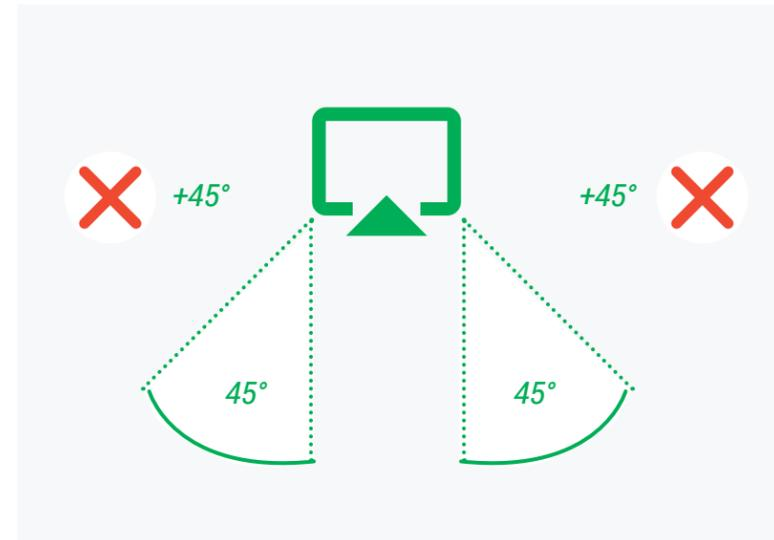
Horizontal viewing angles to video displays should not exceed 45 degrees, measured from the perpendicular of the outer screen edge.
