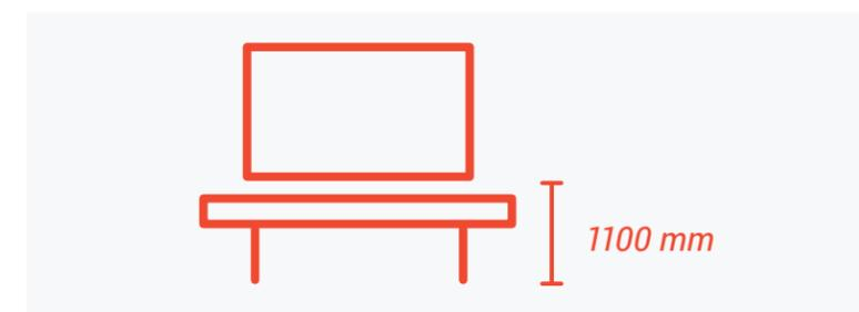
Screens should be mounted centrally to the table. The screen height should allow for comfortable viewing, as a guide keep the bottom of the screen less than 1100mm from the floor.
