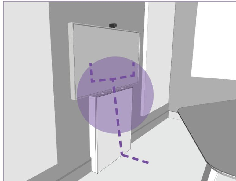
Don't forget to consider cable routes, especially where they might be visible or cause a trip hazard. A conduit or concealed cable route behind the wall to feed the screens will help keep the install neat. If the table doesn't stretch to the wall, then don't forget a route over, or even better under, the floor will be needed.
