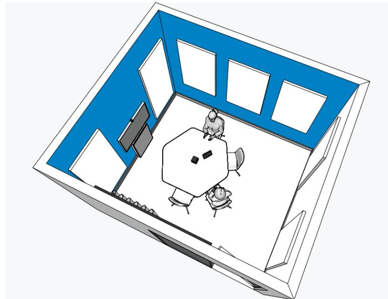
Acoustic treatment on wall areas should ideally feature on two adjacent walls to reduce the risk of parallel reflections forming between two opposite reflective surfaces.
