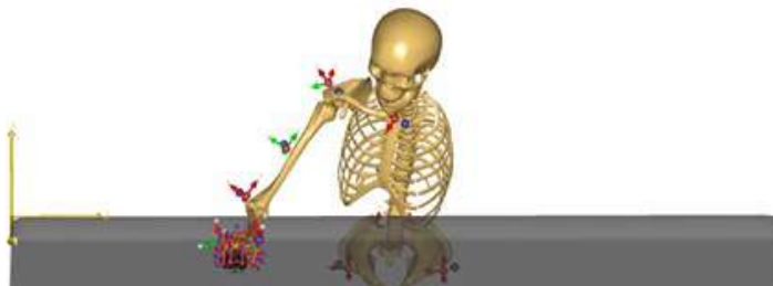
Simulation of Different Centre-of-Gravity Positions Using a Human Musculoskeletal Computer Model
